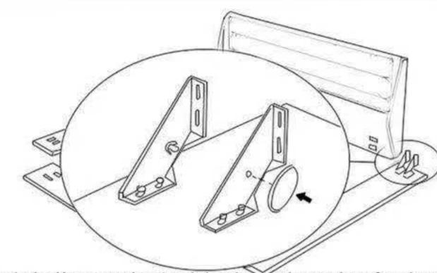
Put the bed legs onto the triangle brackets and paste the soft pads. Attach those 8 triangle brackets onto the 2 sides of the bed. Pleasekeep the bolts and nuts loose and do not tight up at this stage.
